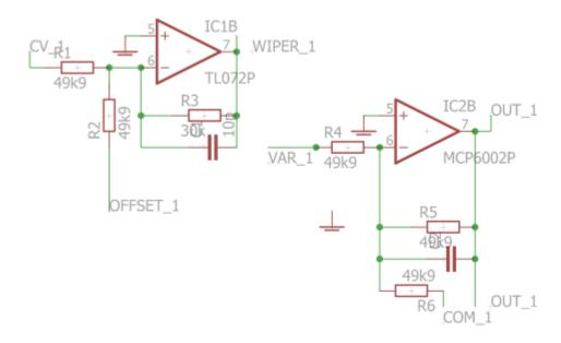
The circuit is a very simple series of two inverting amplifiers per channel. The first is a TL072 powered from +12/-12V, while the second is an MCP6002 powered from 3v3/0V (ground). It's possible to preset the ranges (see below) but it's probably more useful to use the associated Control Board.
