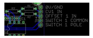
For scaling bipolar CVs, connect or switch into OFFSET (e.g. +5V) For 0-5V operation, leave SWITCH open; for 0-10V operation, jumper or switch in SWITCH
