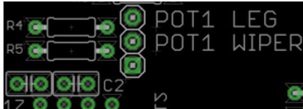
With a 100k pot facing you, solder the left leg to 0V(ground) the centre to WIPER and the right to LEG. WIPER and LEG may be jumpered if pots aren't desired, but it is quite useful to have an attenuator to trim down variable CVs or even clip the second op amp for crunchy waveforms!
