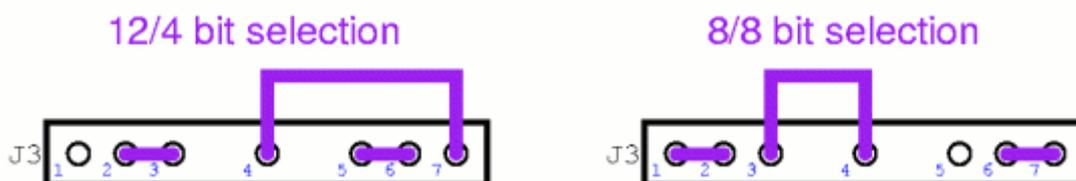
The 12/4 bit option is used by MIDIbox SID (the filter is controlled with 12bit, the resonance with 4bit only). In the MIDIbox CV firmware the resolution option is selectable. 8/8bit is enough if the module should control V/Oct CV inputs via Note or CC events. 12/4bit should be selected if channel #1 is connected to a Hz/V input, or if high-resolution events (NRPNs, PitchWheel) are desired.
