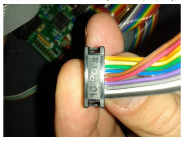
Wire the Core end 1:1 and connect to J19. Note pin 1 is on the bottom left, on the same side as the polarising notch. Take wires 9 and 10 (red and brown in this image) and insert them between wires 4 and 5 (purple and blue in this image). Shift wires 5-8 over so  $5\rightarrow7$ ,  $6\rightarrow8$  etc.
