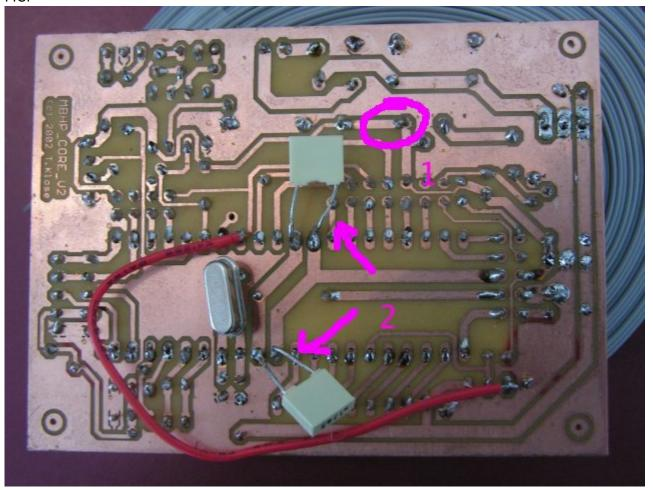
3: This seems to be a bad ground connection directly at the 78xx - it can lead to the wrong voltage. Here the same: just solder the pads again, it will help And same as above: the long cap legs need to be cut, the danger of shorting out is too high!
