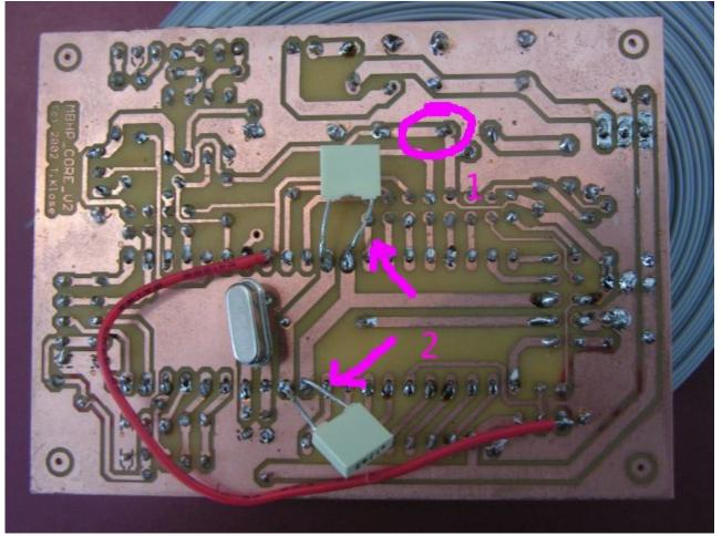
3: this seems to be a bad ground connection directly at the 78xx - it can lead to the wrong voltage. Here the same: just solder the pads again, it will help And same like above: the long cap legs need to be cutted, the danger for shorts is too high! Last update: 2006/12/13 08:39
