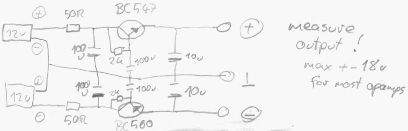
4. What cap size? A standard rule I found in one place is 470  $\mu$ F per 0,1 Ampere. That should be enough. Making the capacitor bigger is no problem (to a certain degree). For our projects I guess 1000 to 3000  $\mu$ F should be absolutely enough. With the single no center tap transformer psu make them twice the size!
