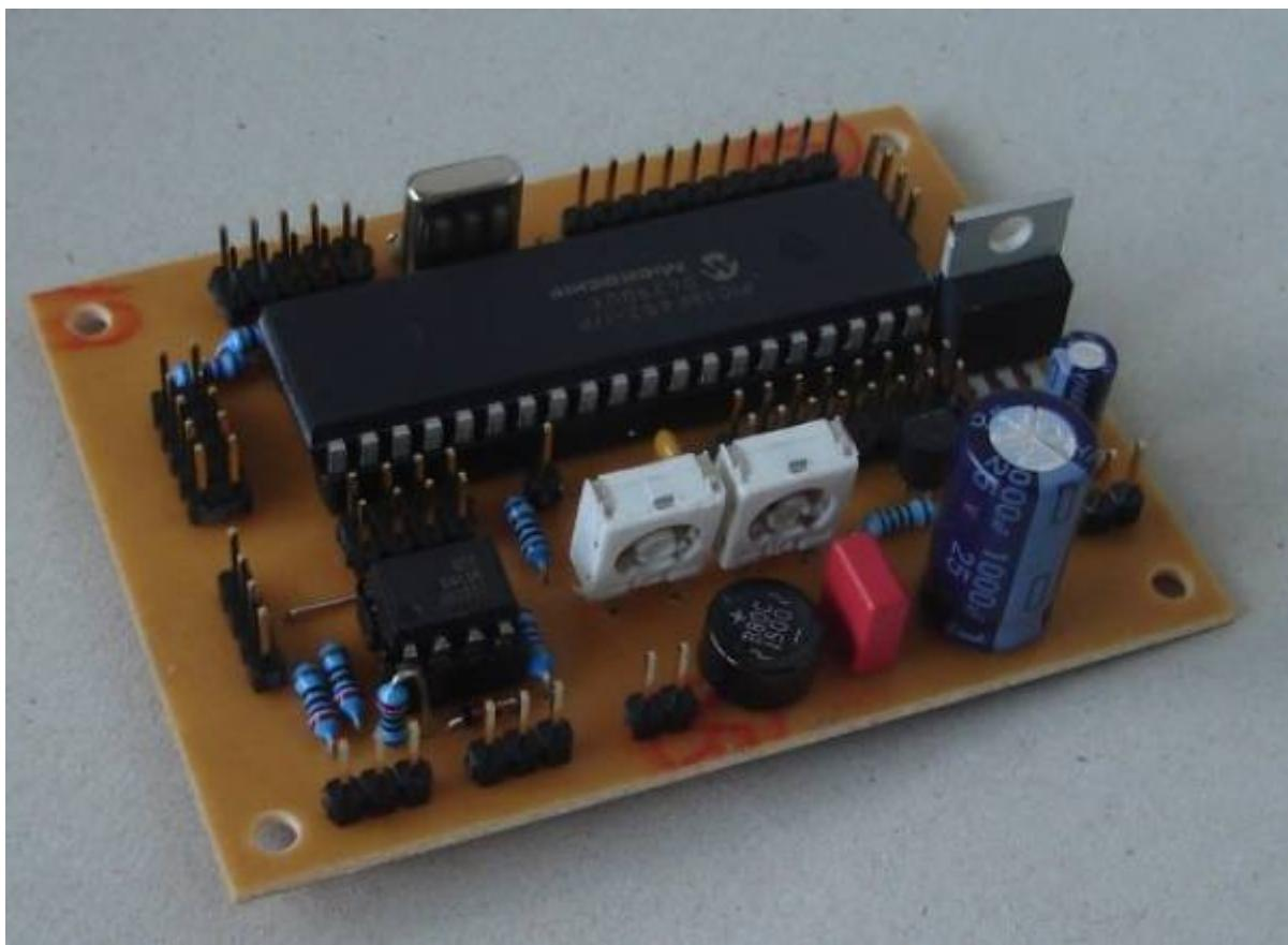
Main part of this module is the PIC18F452, a microcontroller manufactured by Microchip. It is clocked at 40 MHz (externally with a 10 MHz crystal) and offers enough performance to handle analog and digital modules with latencies below 1ms.
