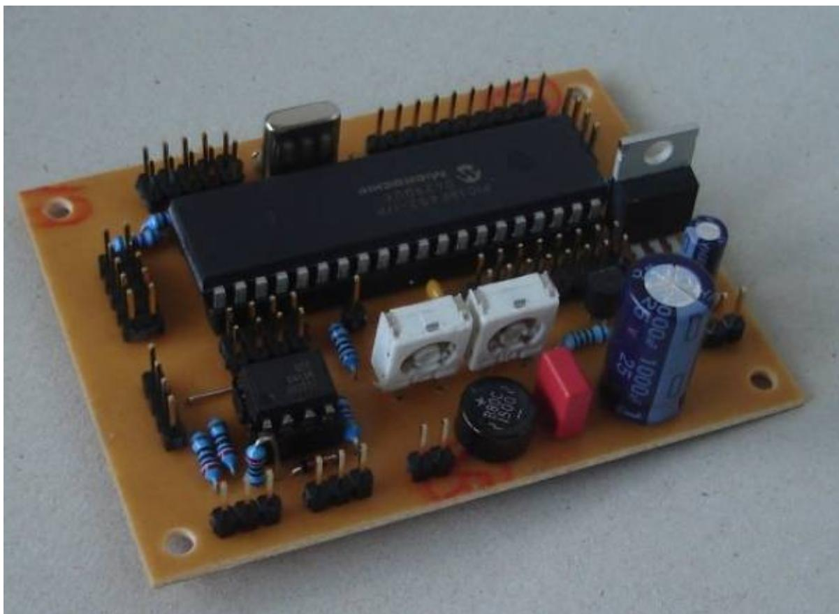
Main part of this module is the PIC, a microcontroller manufactured by Microchip. It is clocked at 40 MHz (externaly with a 10 MHz crystal) and offers enough performance to handle analog and digital modules with latencies below 1ms.
