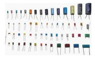
The capacitor is a passive component used to store electrical energy temporarily in an electric field with a value in farads . It is sometimes Polarized (Electrolytic), sometimes not (Ceramic)
