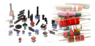
The resistor is a unpolarized passive component with a resisting value in ohms that acts in voltage regulation in circuitry. The color stripes on it describes it value, following a color code
