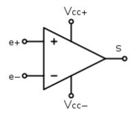
Vcc is the "power supply" voltage for the Operational amplifier
