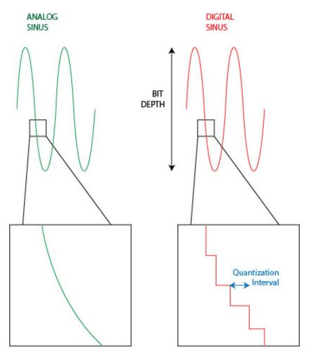
If the numbers representing samples are integers, the quality of the quantization is called the **bit depth**.
