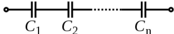
$$(1/C_{\text{Total}}) = (1/C_1) + (1/C_2) + \dots + (1/C_n)$$
