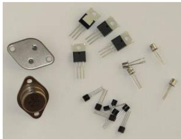
The Transistor is an **active** component that works as an **amplifier** or a **driven switch**.
