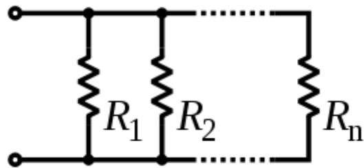
$$(1/R_{\text{Total}}) = (1/R_1) + (1/R_2) + \dots + (1/R_n)$$
