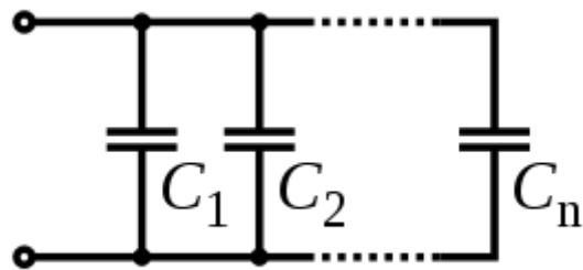
$$C_{\text{Total}} = C_1 + C_2 + \dots + C_n$$
