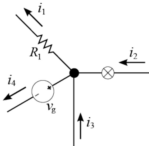
In other words , in a node , Current going to the node equals Current going from the node
