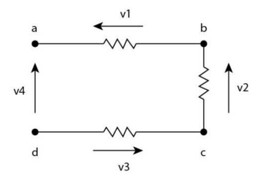
In other words, the voltage is balanced along the components rings; ad = ab + bc + cd
