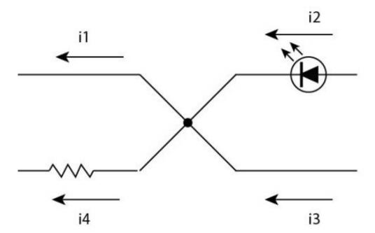
In other words , in a node , Current going to the node equals Current going from the node  $% \left( 1\right) =\left( 1\right) \left( 1\right$
