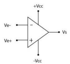
**Vcc is the Bipolar power supply voltage** for the operational amplifier . It is assumed it exists , but not always represented to make things clearer
