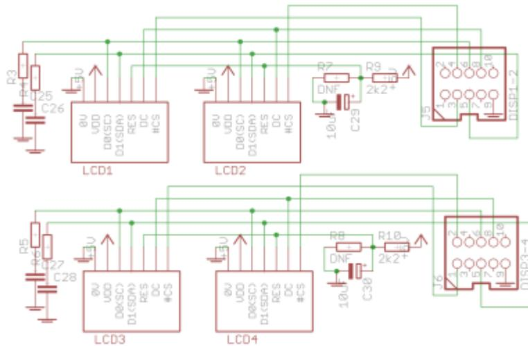
The reset circuits R9/R10/C29/C30 should be installed. The termination circuits R3-6/C25-28 shouldn't be required. When wiring ribbon cables, the end attached to the ELO board should have two IDCs on it; there is no connection on the PCB for the clock/data etc. lines between the two pairs of displays.
