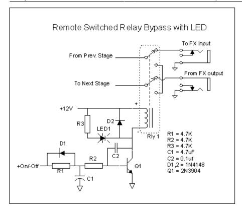
"The neat way to defeat the clicks is to slow down the change in voltage across the inductor. The circuit at left does that. An on/off signal is applied to a resistor/diode/capacitor network on the base of a common 2N3904 transistor. The capacitor to ground slows the on/off transition down on the rising (turn on) edge of the input signal, and the diode lets it turn off fairly quickly.
