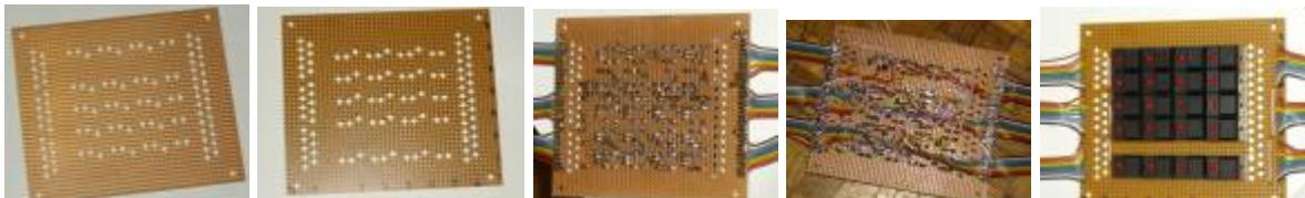
On one side you have the DIN ribbon cables, on the other the DOUT's. On each ribbon cable you have eight of them, one track is a ground. One track stays unused. The connections must match the assignment of the DIL pin-headers for the connection to the DIN/DOUT boards. Note that DOUT's are counted backward for each SR/plug/ribbon cable. See [this](#) page for more information about the issue.
