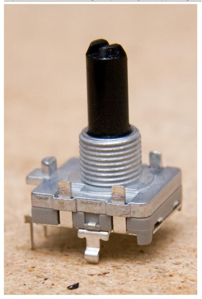
When you open the encoder (might be done using kind of miniature screwdriver or similar), the key to the smooth travel of encoder shaft - is absolute care of the inner circle where collectors travel.
