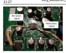
Here the signals are centered around 2.5 volts. After a few experiments I found that these signals are too weak to be fed directly into the LPCXpresso board's ADC inputs, they need some gain. The output signal of the force sensor is captured too, of course the timing requirements are much less demanding here. Here the voltage is taken directly from the force sensing resistor, just via a simple RC low pass filter to suppress noise.
