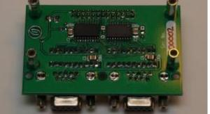
Each I/O Board handles 8 MIDI ins and 8 MIDI outs, i.e. it can connect to up to two BOBs.
