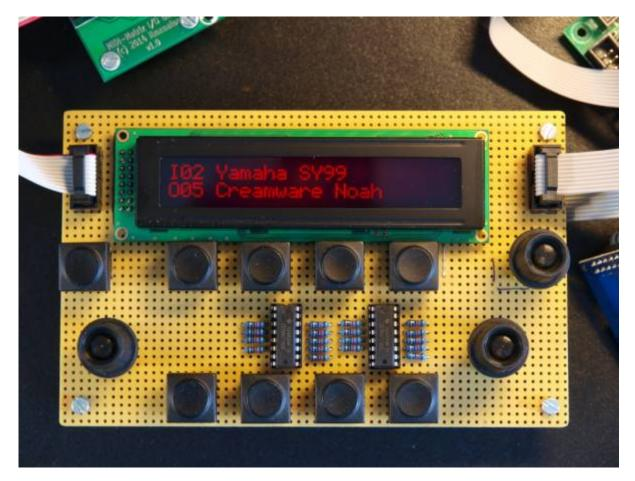
The prototype of the user interface (UI) already shows the main usage paradigm: a rotary encoder (on the lower right) is used to select the out port, thereafter the in port is selected with the rotary encoder on the left. This selection is confirmed by pressing the encoder. More changes to the current routing can be made, and when pressing the lower right rotary encoder, all changes are made effective and the routing is changed.
