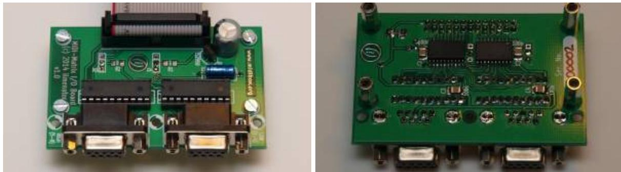
Each I/O Board handles 8 MIDI ins and 8 MIDI outs, i.e. it can connect to up to two BOBs.
