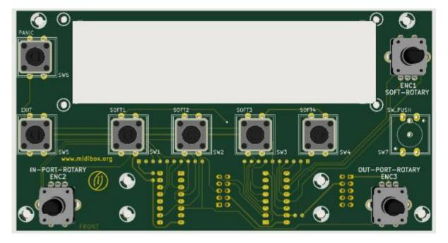
A second generation PCB as modeled above will be ordered soon. This PCB can also be used with other projects involving an SCS, e.g. the MIDIbox NG. Both, my favourite switches from Marquardt (6425 series), as well as the E-Switch TL1100 series (see e.g. MB SEQv4) can be used.
