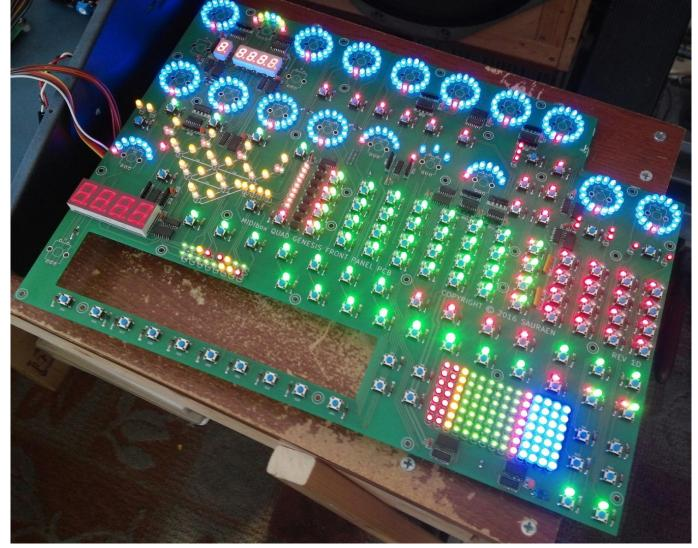
many of each type of LED you will need based on your color preferences and which LEDs will be sticking through the front panel versus lighting up buttons or light pipes. Trust me, you don't want to use regular LEDs to try to light up the plastic, it'll look dim and poor; and you don't want to use the high-brightness LEDs sticking through the front panel, they will blind you!
