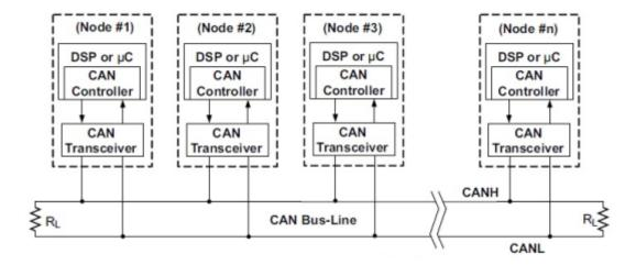
For both connection models, each Node(Device) connected to the buss can transmit or receive data. How is this possible?
