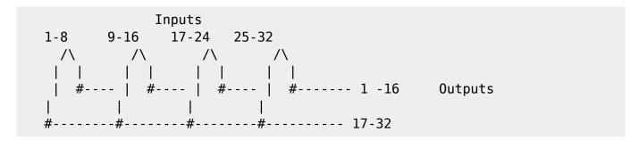
Each set of 8 inputs is split in two and goes to two chips in parallel, so that each set of 8 inputs is capable of being routed to any one of the 32 outputs, which are in two groups of 16.
