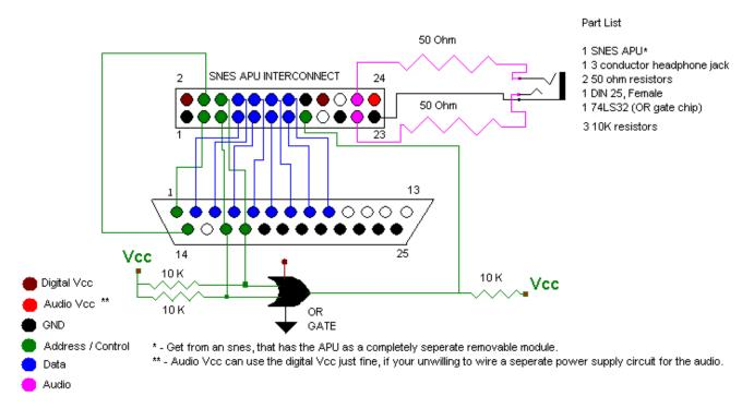
Using this project as an example one can see just how simple getting an APU connected might be. Though I don't have a SNES I can see from this pinout that it's a rather simple task.
