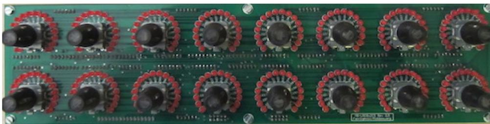
Up to 32 free assignable rotary encoder functions with support for LED rings are available. The encoders have to be connected to a MBHP\_DIN module, the LED rings to four shift registers of a MBHP\_DOUT module.
