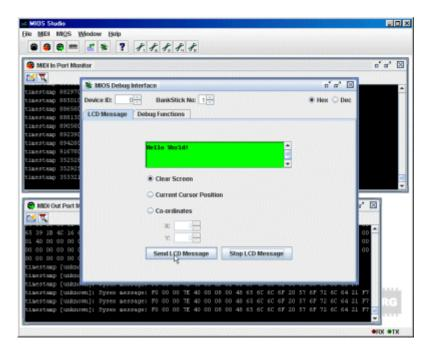
MIOS Debug Functions: The MIOS debug window allows to execute MIOS functions via remote:
