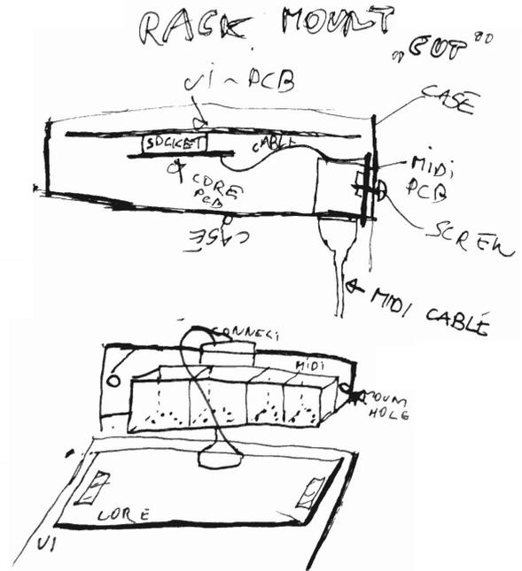
Showing a 10x4cm sized Core32 plugged into a 10x10cm UI-PCB also a midiport-solution is shown, where a midiPCB is fabricated on the core PCB but with the possibility to break it down, the optocouplers diodes and Resistors for the Midiports are on the Core PCB, so the Midi-IO pcb can be small as possibil, so we achive a small Project (small case, small ui...)
