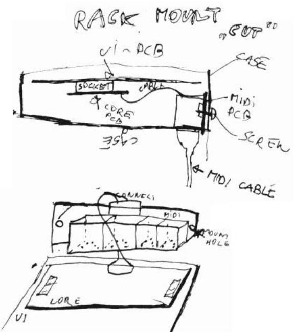
Showing a 10x4cm sized Core32 plugged into a 10x10cm UI-PCB also a midiport-solution is shown, where a midiPCB is fabricated on the core PCB but with the possibility to break it down, the optocouplers diodes and Resistors for the Midipoorts are on the Core PCB, so the Midi-IO pcb can be small as possible, so we achieve a small Project (small case, small ui...)
