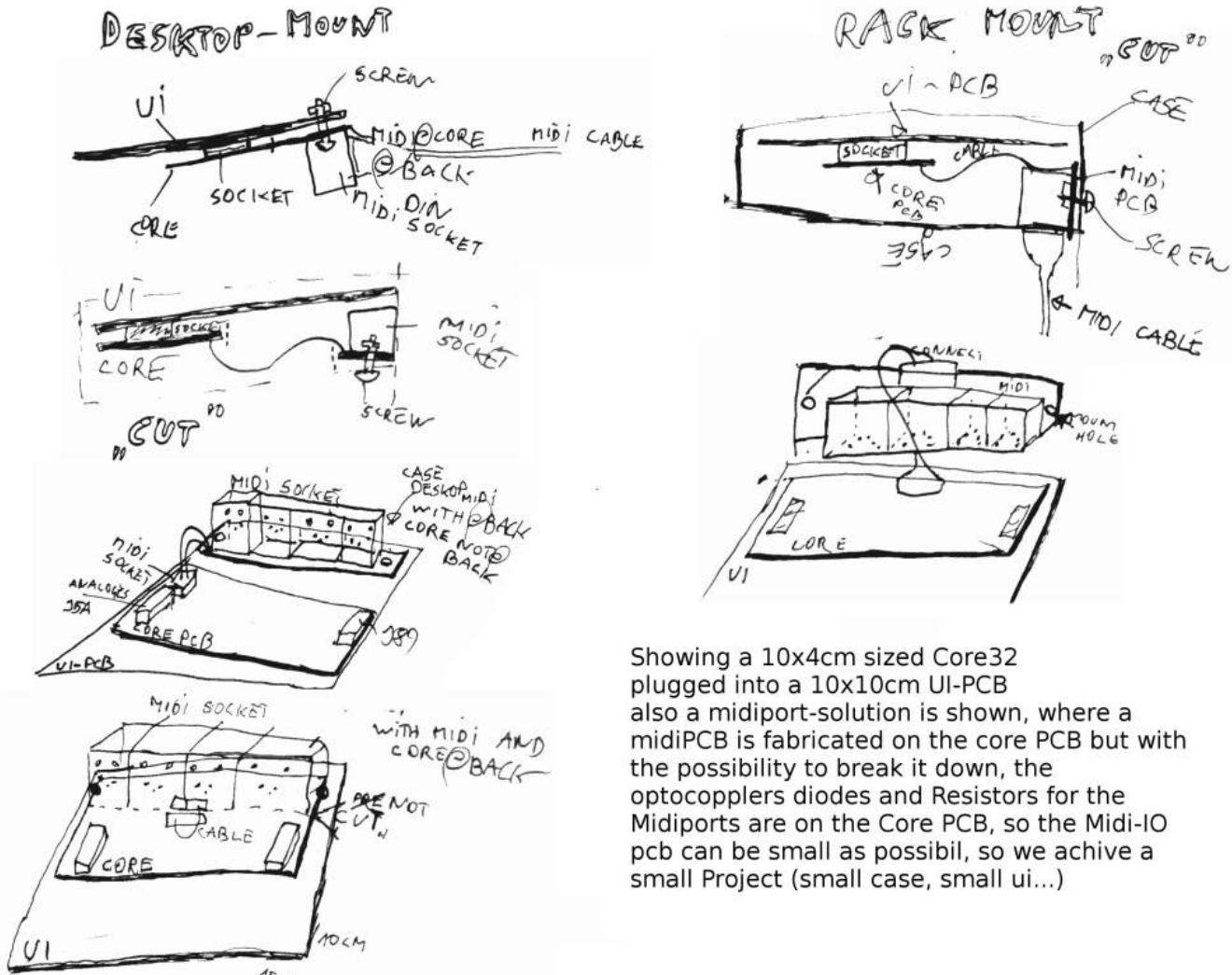
Showing a 10x4cm sized Core32 plugged into a 10x10cm UI-PCB also a midiport-solution is shown, where a midiPCB is fabricated on the core PCB but with the possibility to break it down, the optocouplers diodes and Resistors for the Midiports are on the Core PCB, so the Midi-IO pcb can be small as possible, so we achieve a small Project (small case, small ui...)
