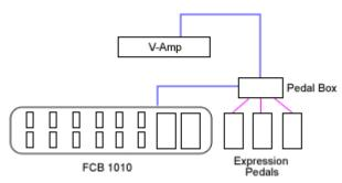
Pedal Box expands your existing floorboard with functionality very similar to Pedal Board Up to 8 Expression pedals and 8 relays can be used. Your floorboard provides the buttons.
