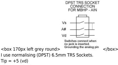
Tip = +5 (vd) Ring = CV (A#) Sleeve = Ground (vs)
