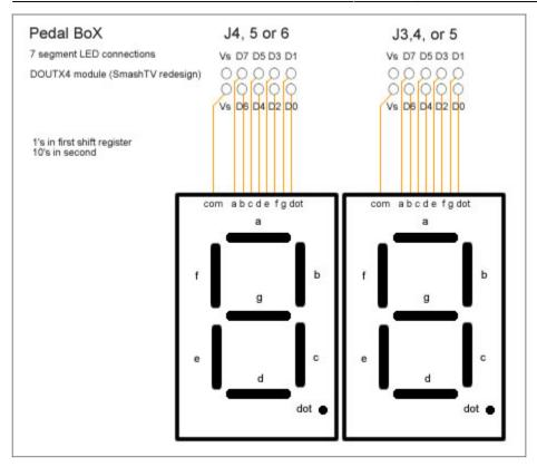
0, 1 or 2 digits can be used (defined in pbx\_config.h). If no digits are used, the current bank is displayed on the LCD (requires a  $2 \times 20$  display)
