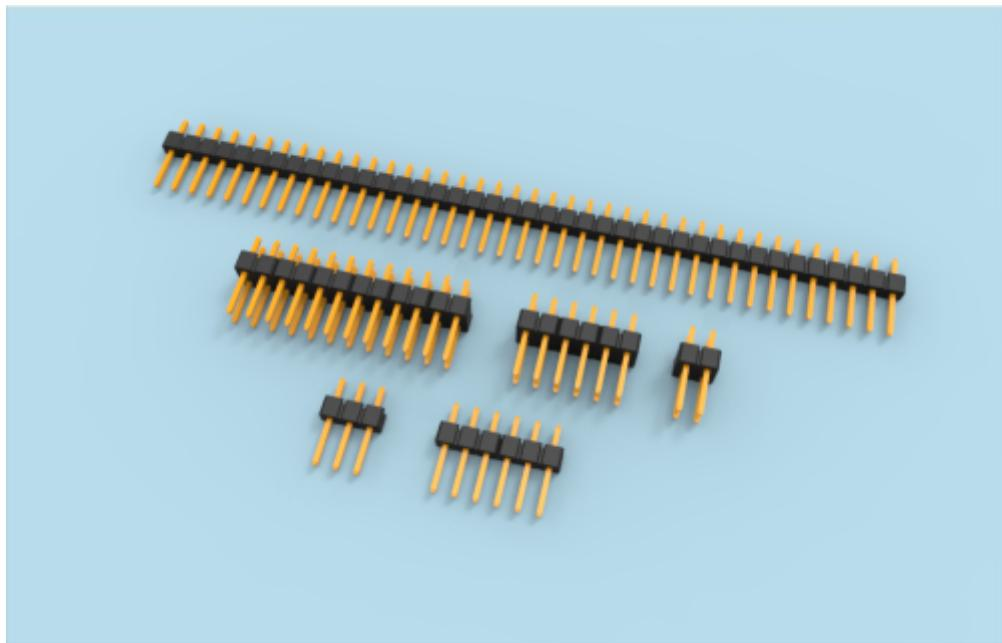
A pinheader is a basic connector to plug things on your PCB without having them soldered. It can be **single or dual row** (SIL-DIL). The usual pitch, aka the distance between 2 pins is 2,54mm. A pin header is designed to be splitted that you can have only the number of pins required to solder.
