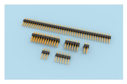
A pinheader is a basic connector to plug things on your PCB without having them soldered. It can be **single or dual row** (SIL-DIL). The usual pitch, aka the distance between 2 pins is 2,54mm. A pin header is designed to be splitted that you can hav only the number of pins required to solder.
