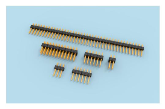
A pinheader is a basic connector to plug things on your PCB without having them soldered. It can be **single or dual row** (SIL-DIL). The usual pitch, aka the distance between 2 pins is 2,54mm. A pin header is designed to be splitted that you can have only the number of pins required to solder.
