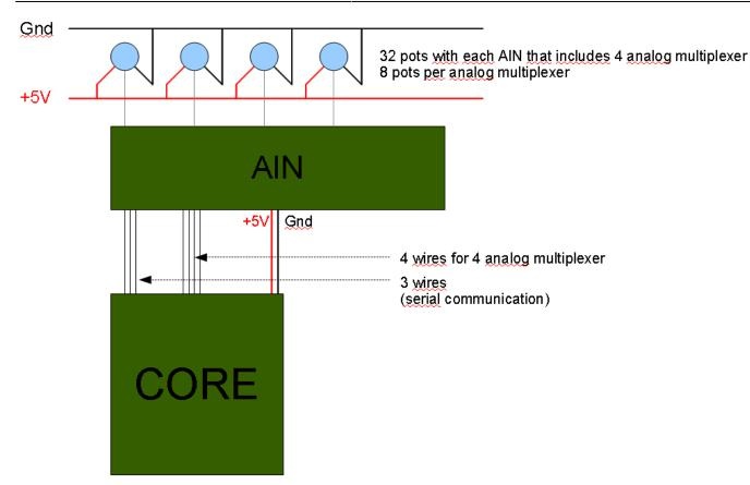
Here is the schematic of all the pots wiring. Each "grey triangle" is a flat ribbon cable with 8 wire on the connector side & only 1 on the other side (the side of the last pots in the row)
