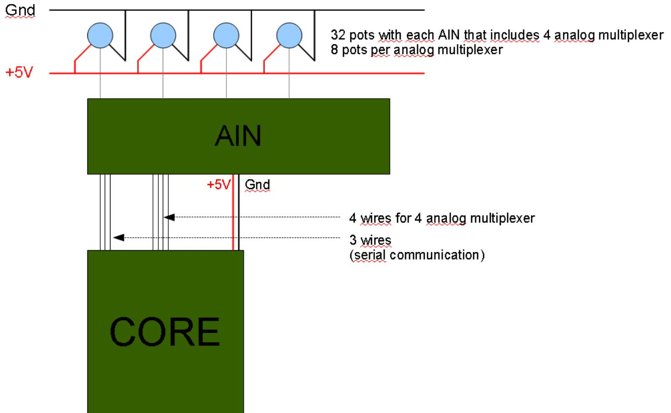
Here is the schematic of all the pots wiring. Each “grey triangle” is a flat ribbon cable with 8 wire on the connector side & only 1 on the other side (the side of the last pots in the row)
