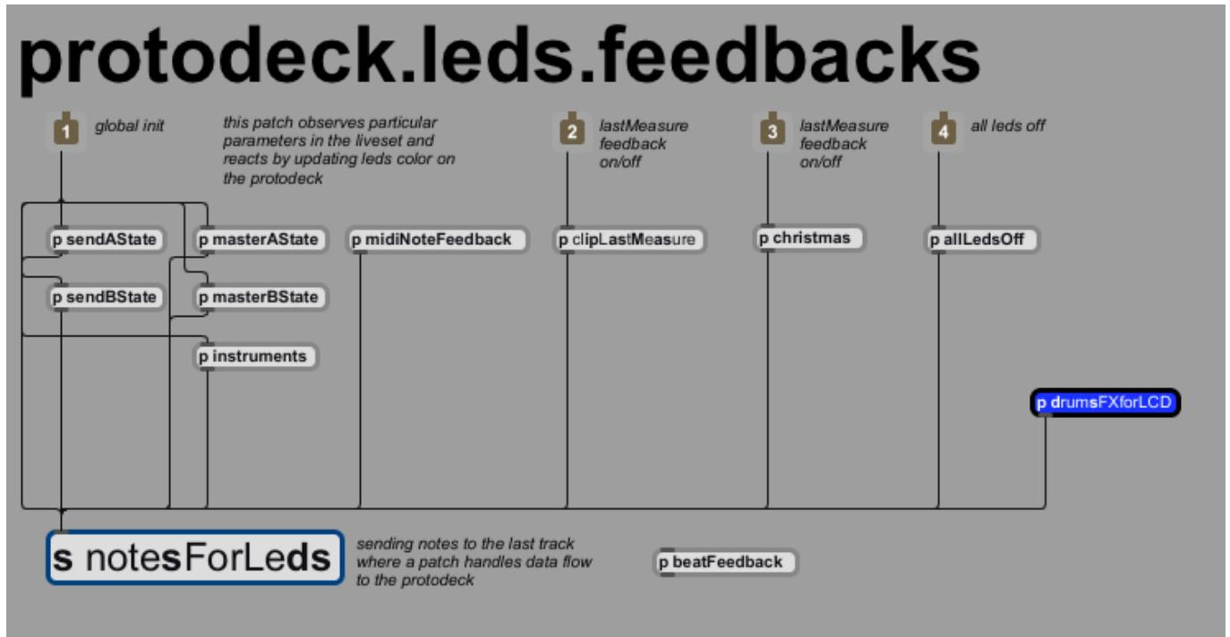
This one handles all the leds feedback, excepted the clip grid feedback (see below with the JS system)
