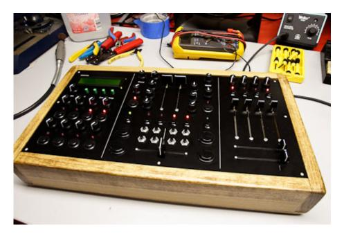
My controller is designed to provide controls for the features I use most in Traktor. Because of this, I've left out controls for features that other users might find essential (looping, pitch control, etc). There is also a section of the controller that is specifically for functions in VDMX, and will not be used for Traktor. In addition to the Midibox controller, VDMX is controlled by a DIY Arduinome (Monome <a href="http://monome.org/">http://monome.org/</a> clone).
