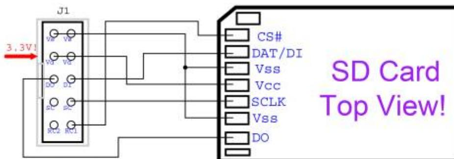
Direct Connections are only possible with MBHP\_CORE\_STM32 (3.3V IO)
