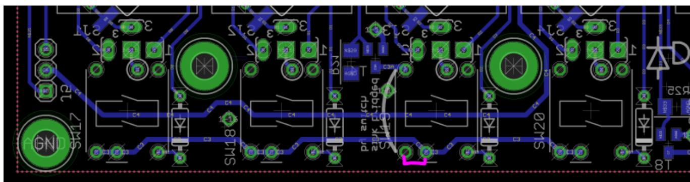
Ghosting. As seems common with these kinds of matrices, there is some unwanted lighting of LEDs. This is most apparent when trying to light up the bottom row of MEC switch LEDs, as the resistive path to the Superflux LED is lower and thus glows unintentionally. This can be overcome somewhat by
