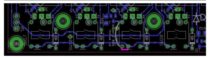
Ghosting. As seems common with these kinds of matrices, there is some unwanted lighting of LEDs. This is most apparent when trying to light up the bottom row of MEC switch LEDs, as the resistive path to the Superflux LED is lower and thus glows unintentionally. This can be overcome somewhat by stacking BAT54 Schottky diodes on top of the BC818 transistors. Later revisions will have more elegant mounting.
