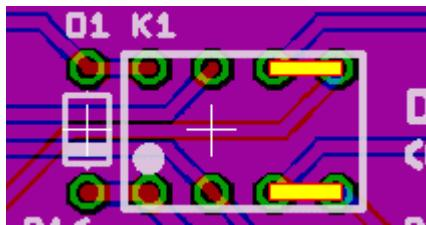
The Omron G6K-2P relay is available at several common places like Mouser, Digikey, Reichelt etc, but is a bit on the expensive side. If space is no issue, you could also use some short wires to solder in a different larger/cheaper/available 12V DPDT relay.
