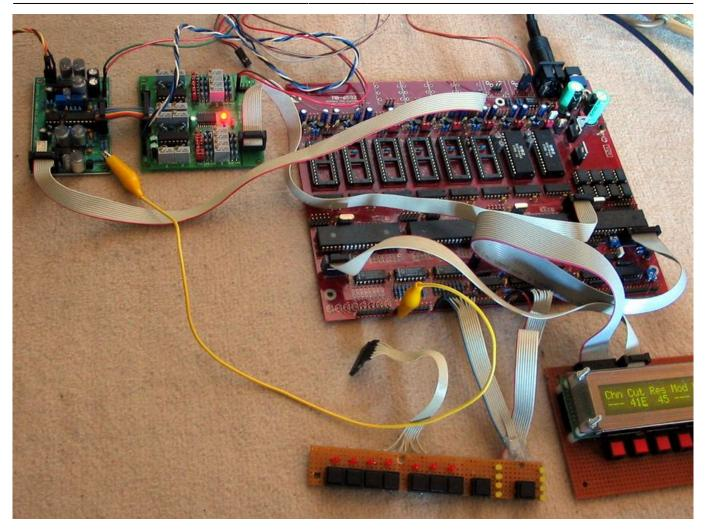
My current test setup, a MBSID V2 (MB-6582 base PCB) with 6581 SIDs and an AOUT NG.
