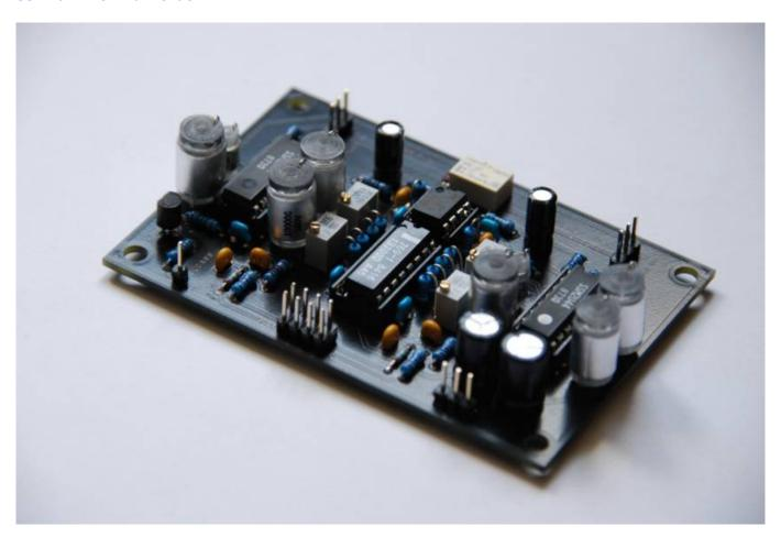
This PCB contains two of the famous SSM2044 24dB low pass filters with the necessary circuitry, additional LM13700 based Q linearization circuit and a tiny Omron micro relay for a software controlled (via gate out pins) bypass function. The layout is optimized for use with the AOUT\_NG module, requiring the addition of a bipolar option when used with regular V/Oct sources like the original AOUT module.
