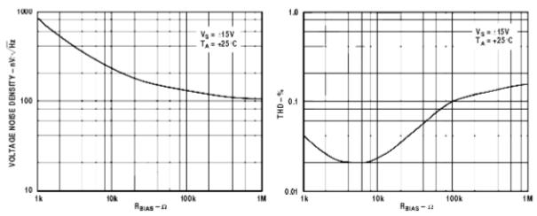
Figure 11. Voltage Noise Density vs. R<sub>BIAS</sub>
