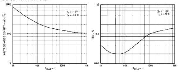
Figure 11. Voltage Noise Density vs. R<sub>B(AS</sub>
