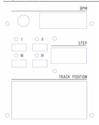
The cutouts for the 7-segment displays and the LED matrix modules hold little plexiglass windows that I had also made at Ponoko. I have access to a (manual) milling machine, so I milled a groove surrounding each cutout on the backside of the panel. The plexiglass window has an identical groove on the front so that the two sit flush and can be glued together quite easily. You probably don't need the two inner mounting holes (above and below the STEP display) at all.
