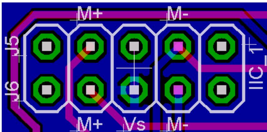
this is the midi i/o header for the iic modules. J5 is midi input and J6 is midi output.
