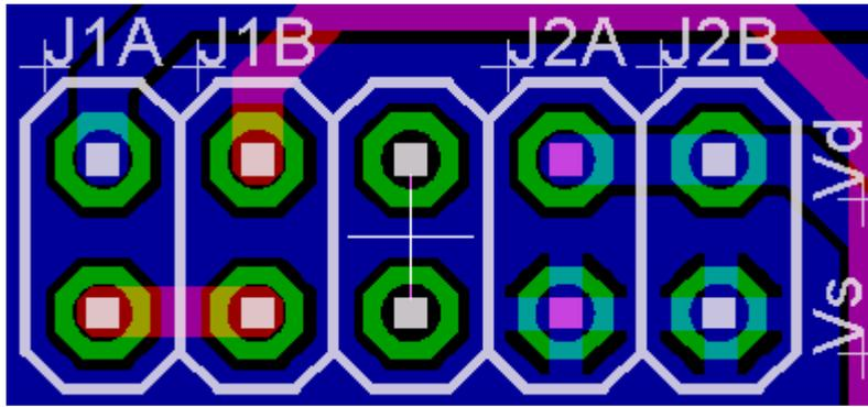
J1A is a connection to your power supply, and J1B breaks the connection to the core to allow for a switch. to bypass the switch, simply insert a jumper into J1B or connect the top pins of J1A and J1B to the power supply.
