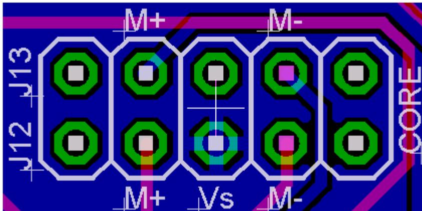
this is the midi i/o header for the core. it uses a 6 or 10 pin dil header. this configuration was requested on the forum. i am using this with a pair of 3-pin sil connectors from futurlec and they sit very snug on the header. J13 is midi input and J12 is midi output.
