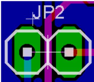
JP2, JP3, and JP4 configures the pcb to be used as a router. connect each set of pins together if you're using a router. leave them disconnected for a seq.
