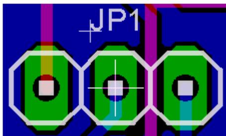
JP1 configures the pcb to be used as a seq or a router. for seq, connect the left and center pins. for a router, connect the right and center pins.
