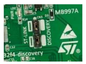
Note that pin 1 of the 6-pin SWD interface on CN2 of the Discovery board only **detects** the voltage of the target. Thus the most foolproof method of flashing is to connect a mini USB cable to the 407v board and set the power switch to USB. This ensures that the board is always powered up when programming. After the bootloader is burned in, the 407v board can be installed in the wCore PCB through the two 2\*25 headers.
