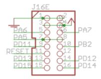
The original J16 functionality is preserved, but extra pins are available on a IDC16 header. These include the Reset signal and pins normally controlling LEDs. This header is normally connected to the RES-SD module.
